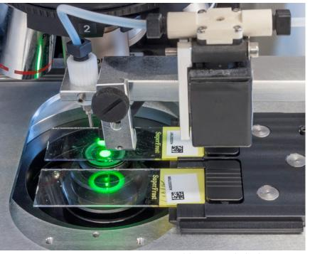
Immersion oil dispenser attached to the microscope
